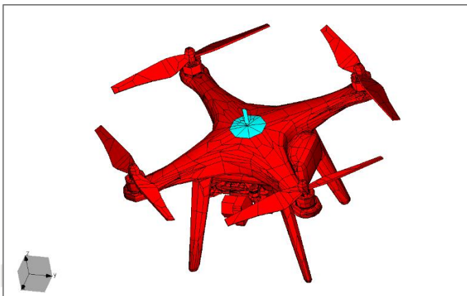
Figure 1. Meshed model of the drone with the monopole and the payload in WIPL-D Pro
