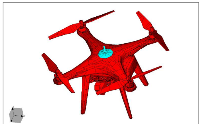
Figure 2. Meshed model of the drone in WIPL-D Pro
