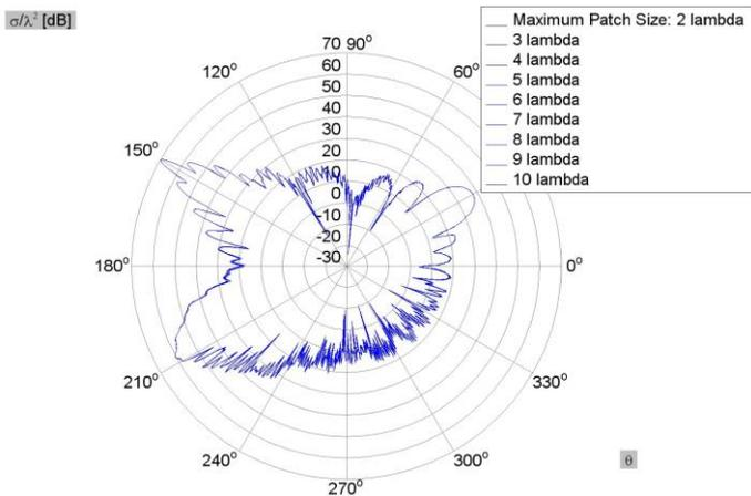
Fig. 8. RCS for various maximum patch sizes.
