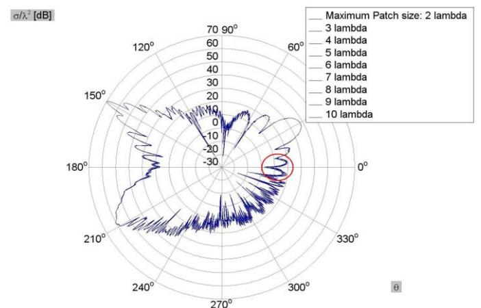
Fig. 6. RCS for various maximum patch sizes
