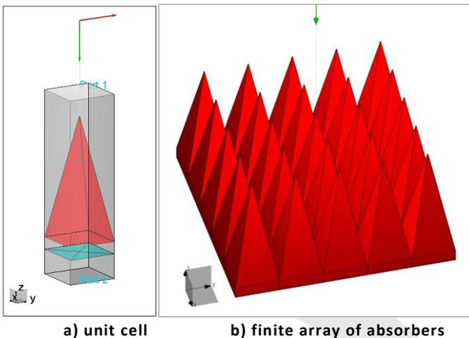
**Fig. 2. Pyramidal absorber**
