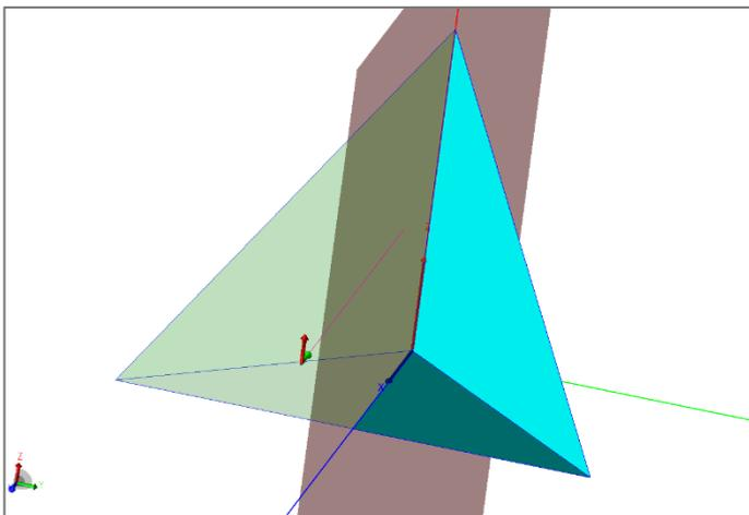
Figure 1. WIPL-D Pro CAD model of the corner reflector.
