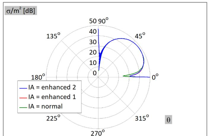
Figure 5. RCS obtained in polar coordinate system for IA set to *enhanced 2*, *enhanced 1*, and *normal*.
