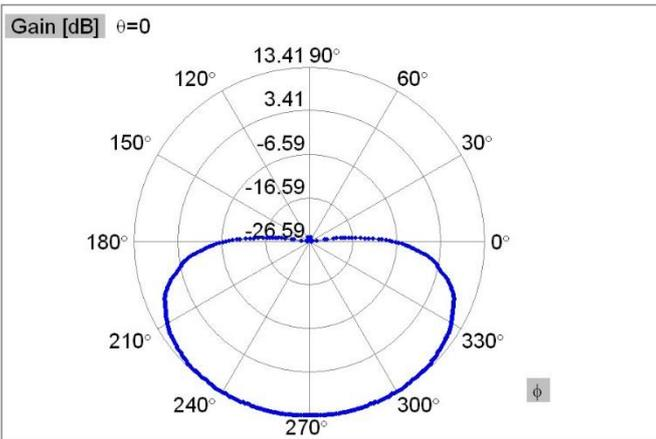
Figure 4. Pattern in two principle planes at 24 GHz
