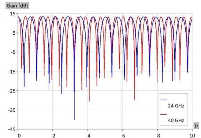
Figure 6. Comparison of pattern for small elevation angles for 2 operating frequencies
