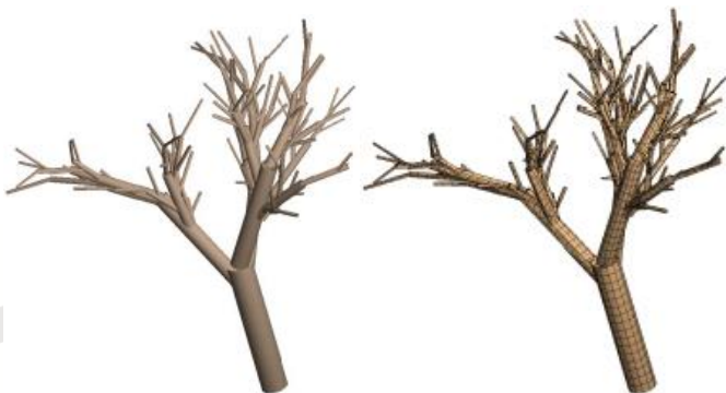
Fig. 4. Wire model and corresponding dielectric model
