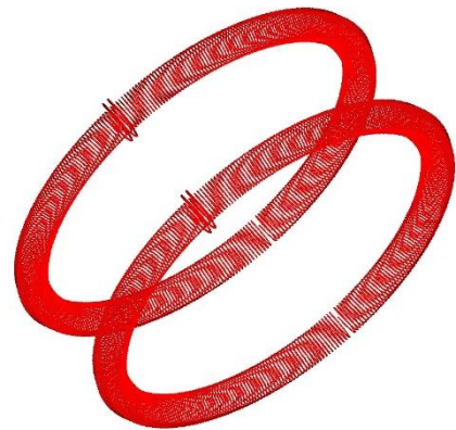
Fig. 4. Toroid coil – wire model.
