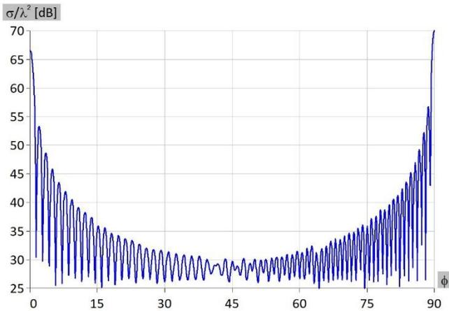
Figure 7. Monostatic RCS from the PEC cuboid
