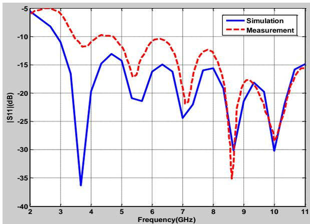
**Figure 10. Vivaldi in free space return loss compared to the measured data**
