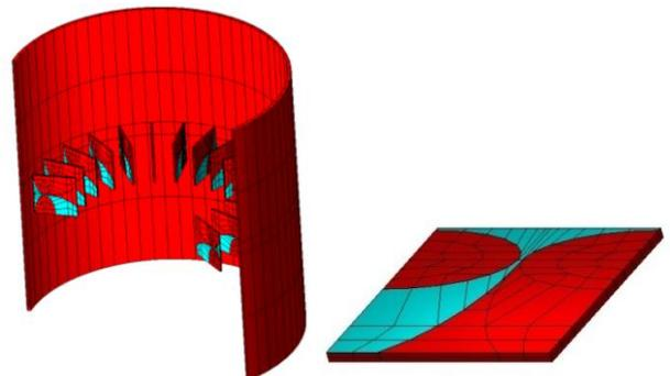
Figure 9. WIPL-D simulation and single Vivaldi antenna
