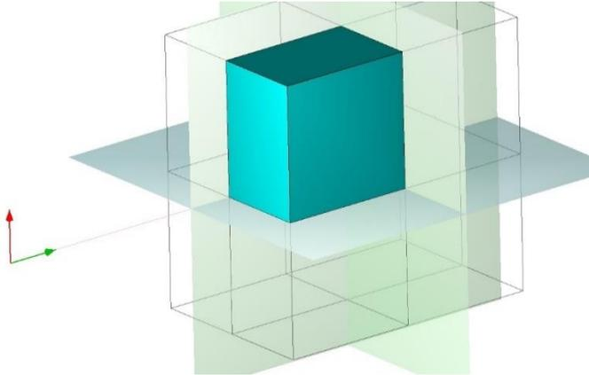
Figure 6. PEC cuboid with 3 symmetry planes
