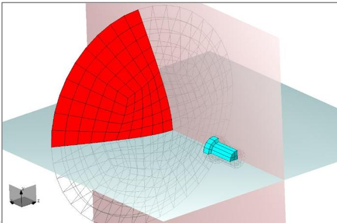
Figure 1. Hyperboloid lens with choke horn antenna
