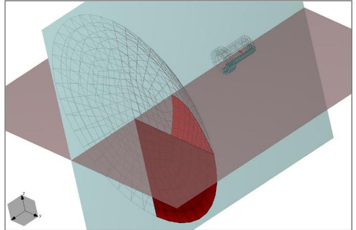
Figure 2. Hyperboloidal lens with horn – rotated preview
