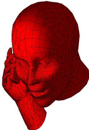
Figure 5. Meshed human head model with mobile phone
