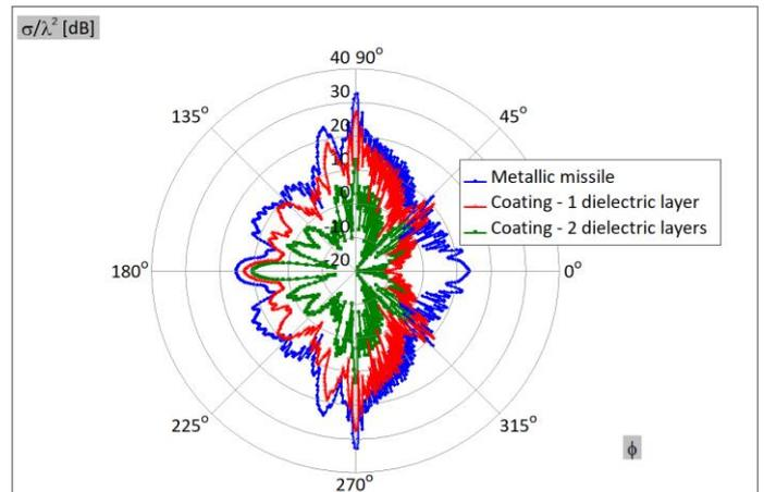
Figure 3. Metallic missile and coated missiles - scattering
