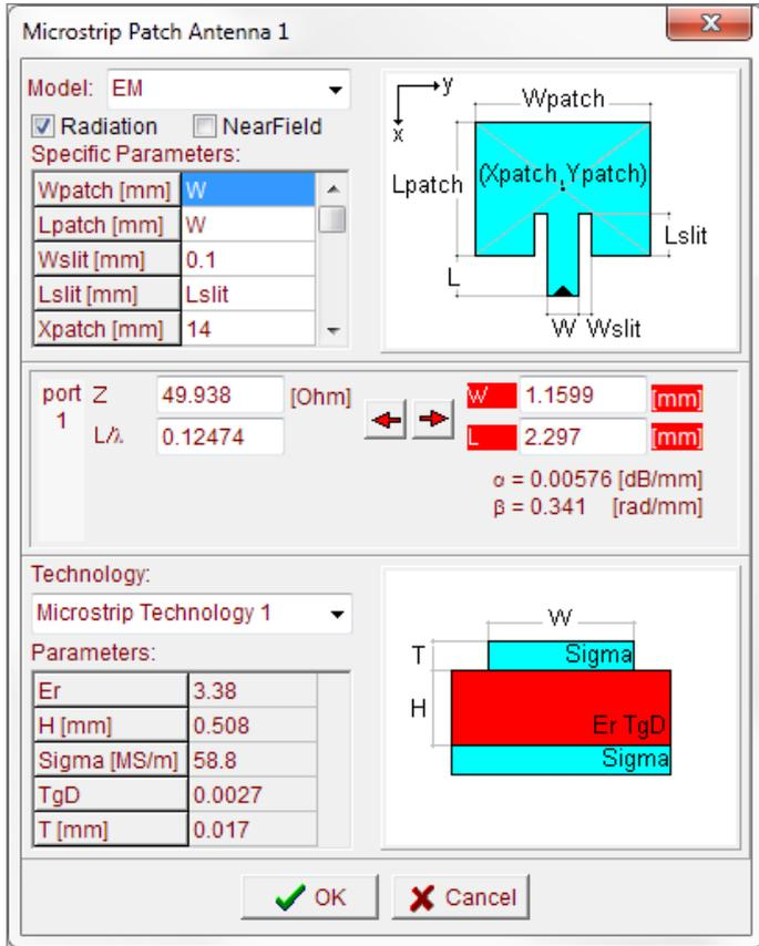
Figure 3. Library microstrip patch antenna model
