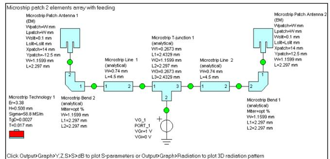
Figure 1. MW circuit
