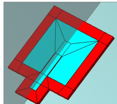
Figure 2. Full-wave microstrip patch antenna model
