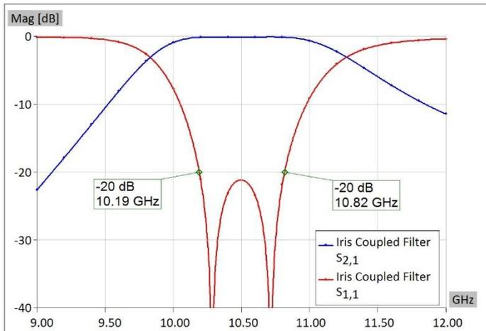
Figure 4.  $S_{11}$  and  $S_{21}$  parameters- simulated iris-coupled waveguide filter
