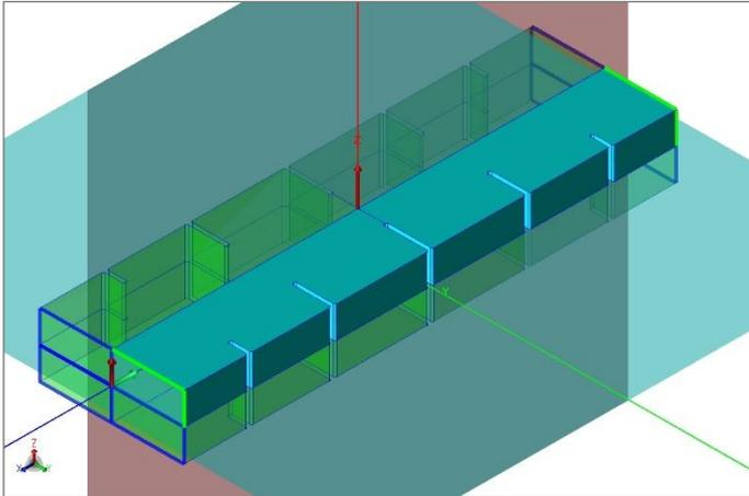
Figure 1. Iris-coupled waveguide filter in WIPL-D Pro CAD
