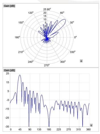
Figure 2. Simulated radiation pattern
