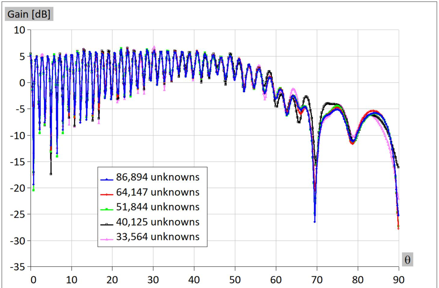
Figure 2. Influence of appropriate smart reduction on radiation pattern
