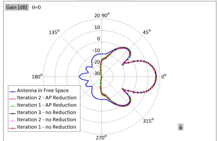
Figure 5. Radiation patterns of the anti-collision radar antenna in free space and anti-collision radar antenna mounted on the bumper
