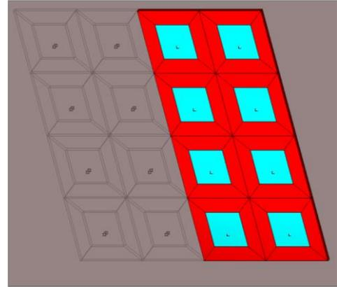
Figure 1. Anti-collision radar antenna – WIPL-D Pro
