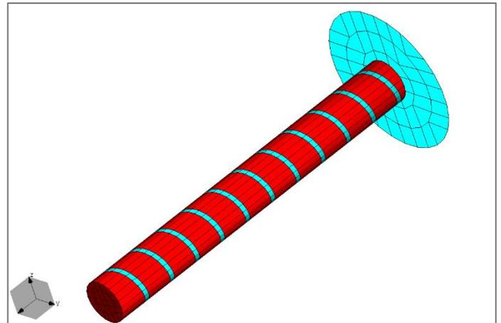
Figure 3. Plate helix with dielectric support
