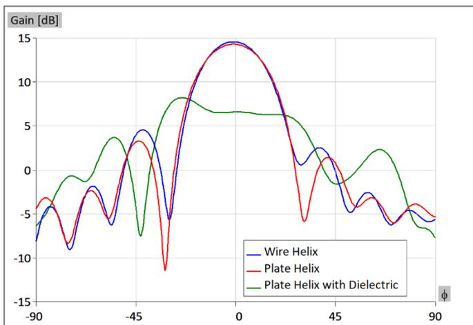
Figure 5. Radiation patterns-wire helix, plate helix and plate helix with dielectric support
