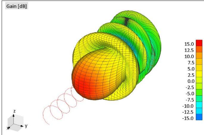
Figure 4. 3D Radiation pattern-wire helix antenna
