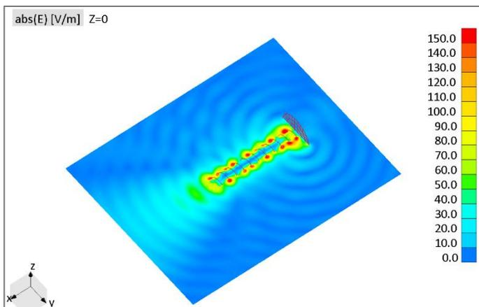
Figure 6. Near field distribution-wire helix antenna
