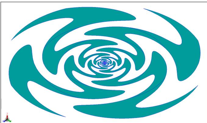
Fig. 6. Four arm sinuous antenna.
