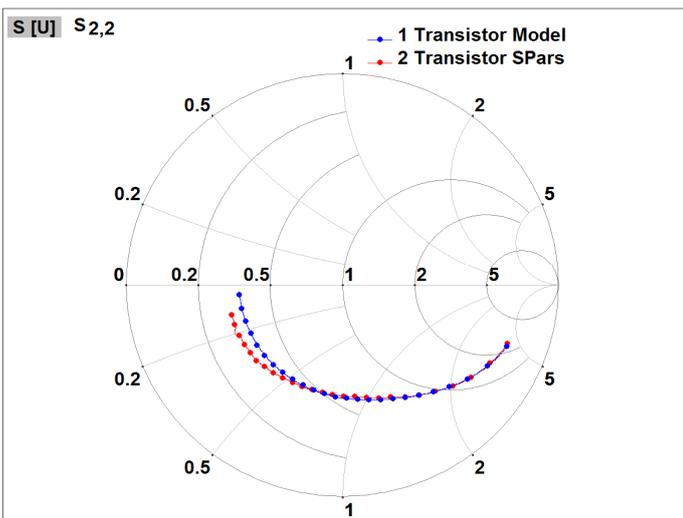
Figure 9. Comparison of S22 parameter of a HEMT device obtained by equivalent circuit model simulation and as listed in a datasheet.
