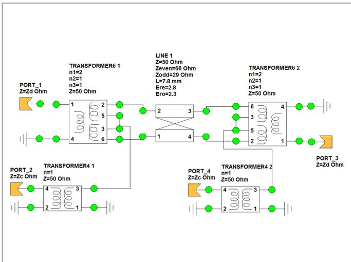
Figure 5. Differential and common mode analysis by using transformer schematic elements.
