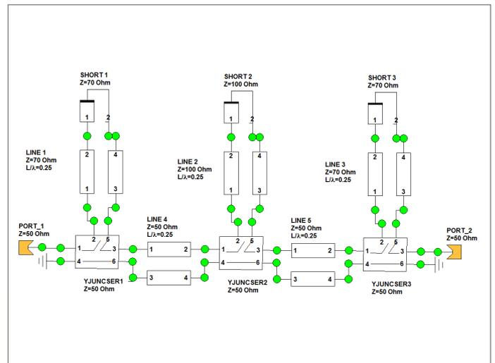
Figure 7. Band stop filter realized with floating ground components.
