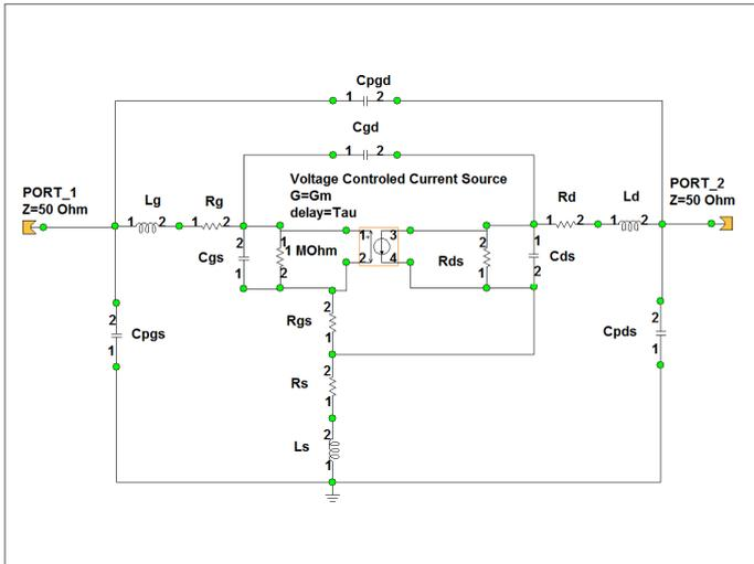
Figure 8. HEMT model utilizing voltage controlled current source with delay.
