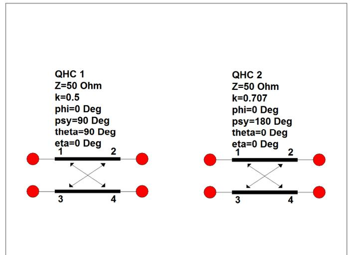
Figure 6. General coupler element configured as quadrature (on the left) and antiphase (on the right) coupler.
